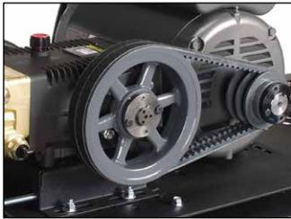
■ Industrial-strength **Motor** and cast-iron, bushing **Pulleys** use a convenient 2-bolt pulley adjustment for easy maintenance and longer life; notched, heat-reducing, "V" cogged belts connect the motor to the rugged **High-Pressure Pump** with three ceramic plungers, a forged brass head and a unique design that results in lower RPM than comparable pumps for less maintenance and a longer life. The pump also is backed by a 7-year warranty.
