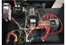
PROGRAMMABLE SMART CONTROL now standard for all VNG machines allows auto start/stop and time delay shutdown features without changing any hardware. It also provides complete control of the equipment run time.
